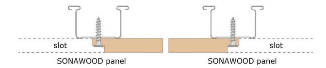
3mm min. gap typical between panels in both directions
