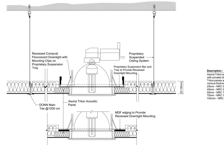
Asona Triton acoustic panel with sonatex facing. Triton panels available in various thicknesses 25mm - NRC 0.75 40mm - NRC 0.90 50mm - NRC 1.00 75mm - NRC 1.00 100mm - NRC 1.00
