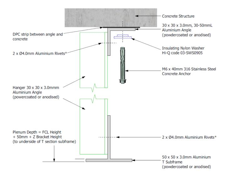
\*Refer Section 3, Components for full rivet specification
