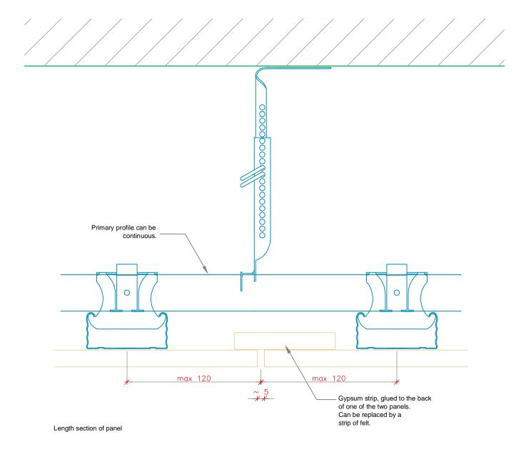
Where expansion joints are present in the primary constructions, the suspended ceiling construction must be correspondingly interrupted!
