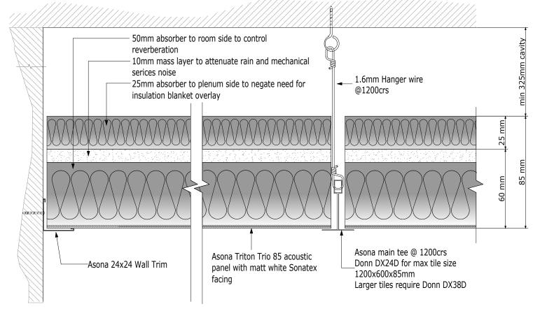
For standard panel dimensions: 600x600x85mm with grid Donn DX24D / DX38D 1200x600x85mm with grid Donn DX24D / DX38D 2400x600x85mm with grid Donn DX38D Title:
